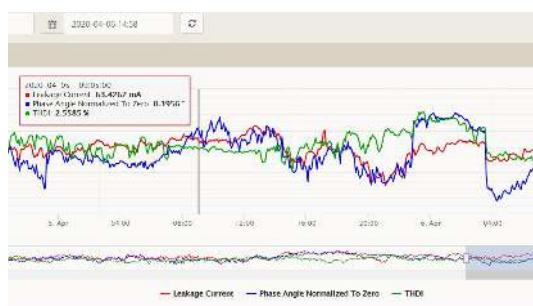
Intuitive user interface showing bushing power factor, capacitance and harmonic distortion.
