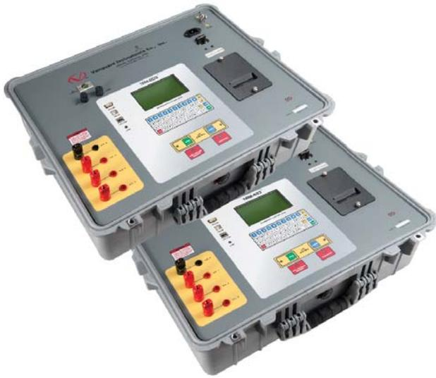
The TRM-203 and TRM-403 are three phase transformer winding resistance meters that allow the user to connect all test cables to the transformer bushings. The unit will then measure the transformer resistance value for each of the phases without the need to disconnect and reconnect cables for each phase.
