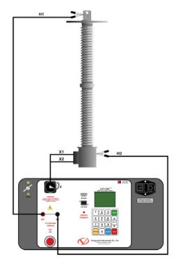
The CVT-765 can measure the turns-ratios of Capacitor Voltage Transformers ranging from 75 to 15,000. The measured turns-ratio, winding polarity, and winding phase angle are displayed on the unit's LCD screen.
