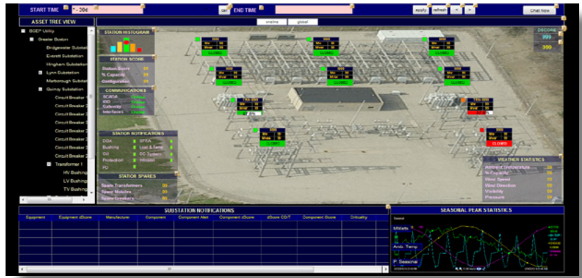
dobleARMS™ offers traditional one-line and geospatial views of asset condition within the substation with links to drill down to asset views.
